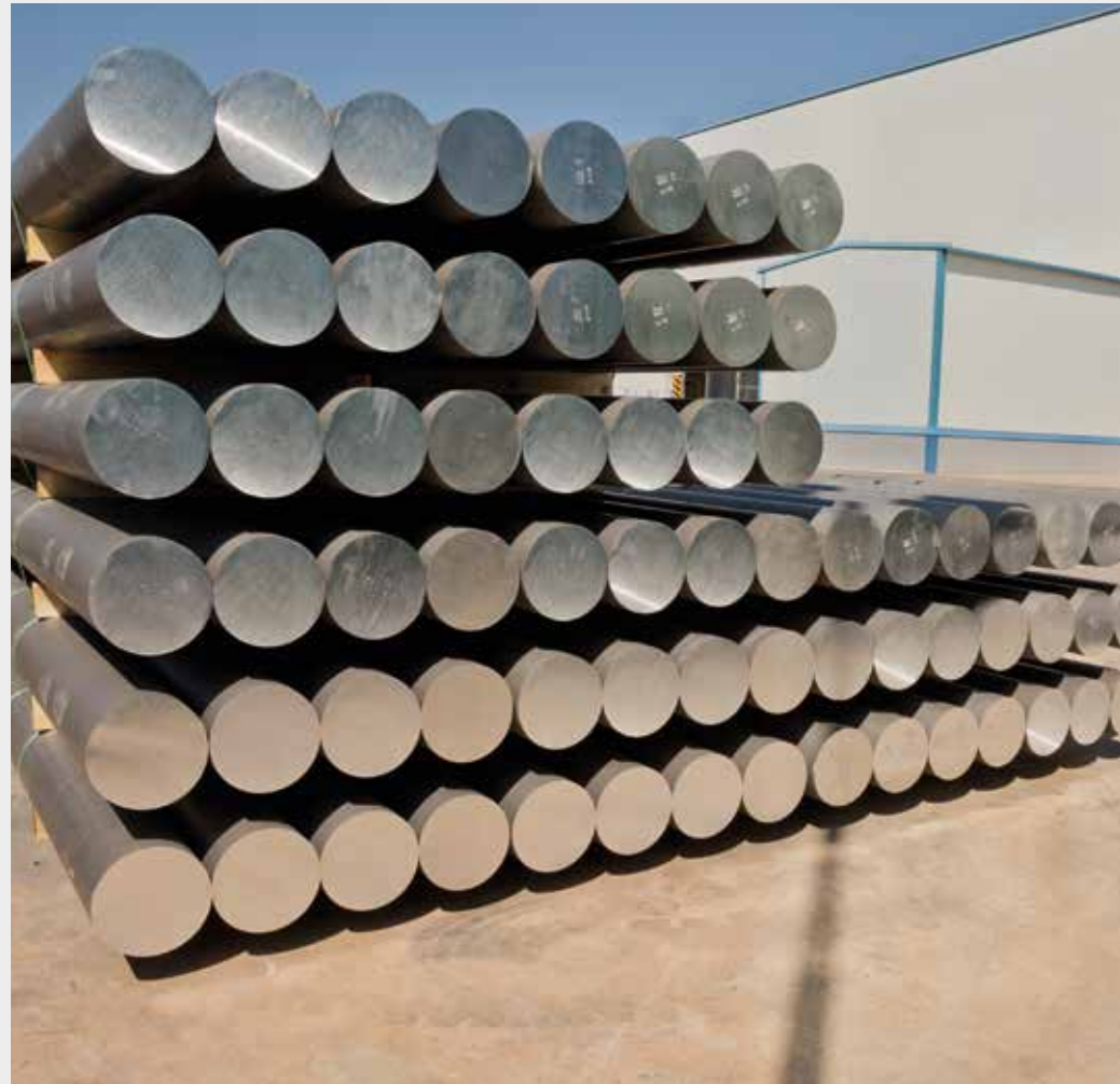
Cylindrical ingots also called "billets", to obtain straight aluminium profiles and eliminate any tension in the material, they are stretched. They are then cut into suitable lengths and artificially aged to achieve the appropriate strength.
